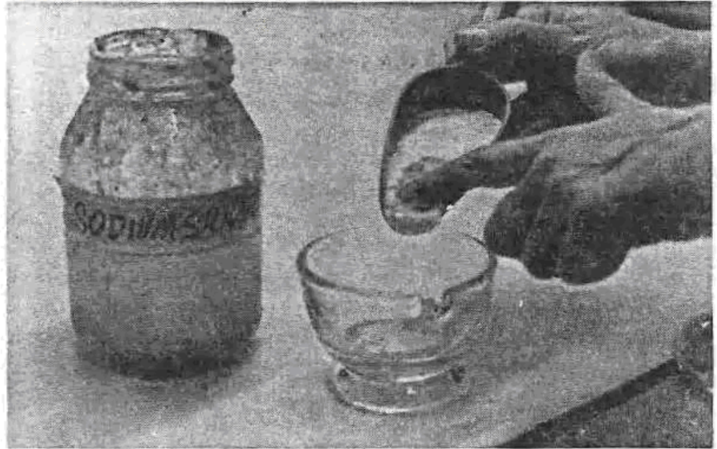
Sodium silicate was used to mix with dry glaze.
