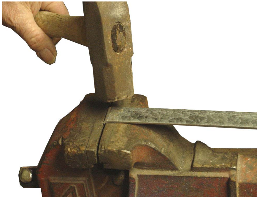
Figure 5 Hammering the bend.
